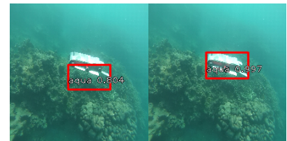
Figure 2. RetinaNet bounding box predictions pre-augmentation (left) and post-augmentation (right).
